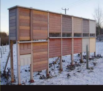
LOW MAINTENANCE TRANSLUCENT FINISHES ARE PARTICULARLY DESIRABLE, YET DIFFICULT TO ACHIEVE ON TIMBER CLADDING AND JOINERY. THIS STUDY DEMONSTRATES ACCOYA COATED WITH A TEKNOS TRANSLUCENT SYSTEM PROVIDES A LOW MAINTENANCE OPTION. THIS SUBSTANTIALLY EXCEEDS THE PERFORMANCE OF TRADITIONAL TIMBER TYPES,
