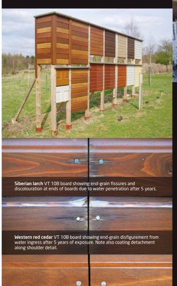
$\begin{tabular}{ll} \bf Accoya \ VT \ 10B \ board \ showing \ no \ end \ fissuring \ or \ discolouration \ from \ water \ ingress \ after \ 5 \ years \ of \ exposure. \end{tabular}$
